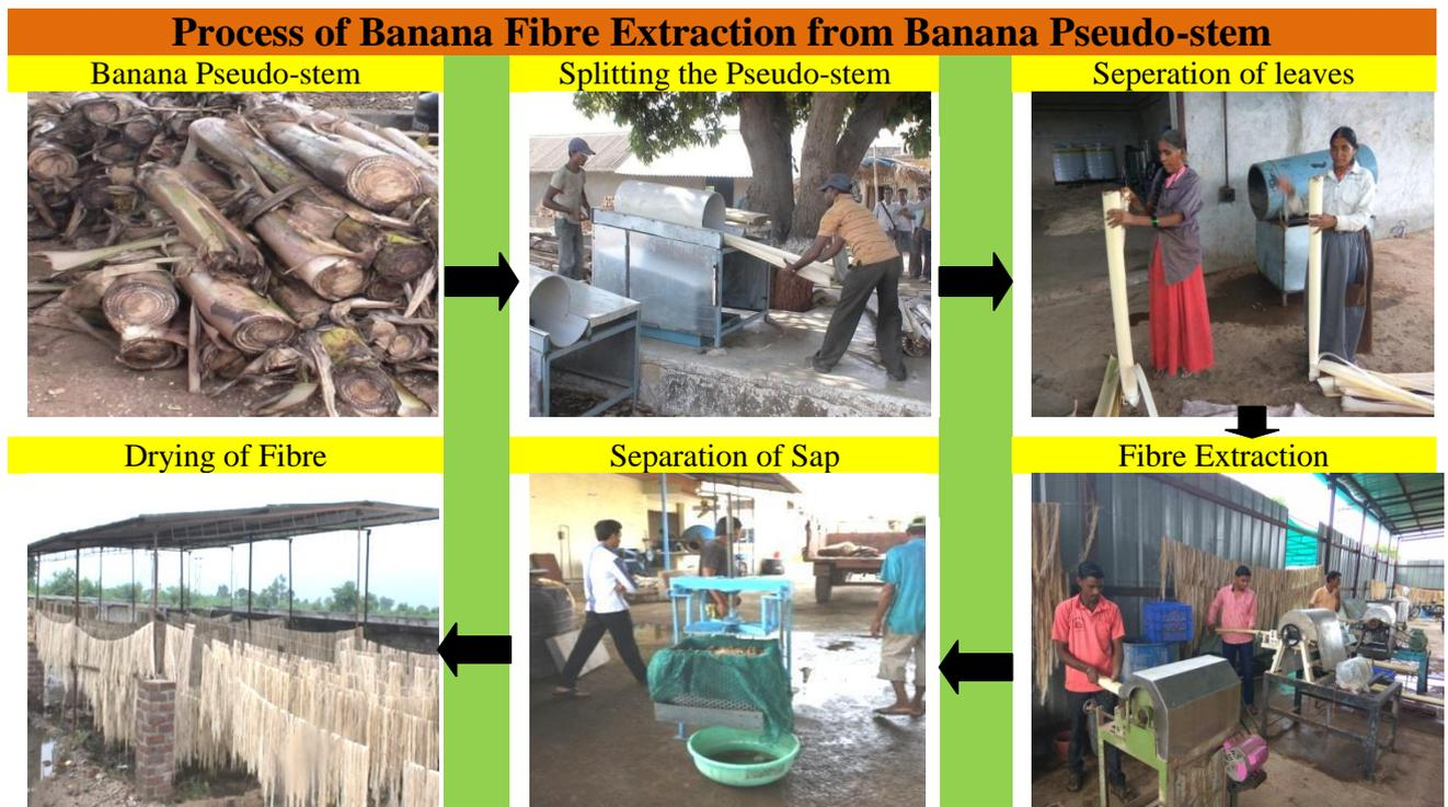
Single Fibre Extraction Machine can extract around 15-20 Kg. of banana fibers per day from 1 MT of pseudo-stem (approximately 50 to 60 nos. of pseudo-stem), to achieve maximum utilization of available pseudo-stems large number of units need to be established across the banana cultivation area.
